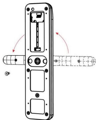
2.The direction of the rear panel handle is opposite to the front panel handle
